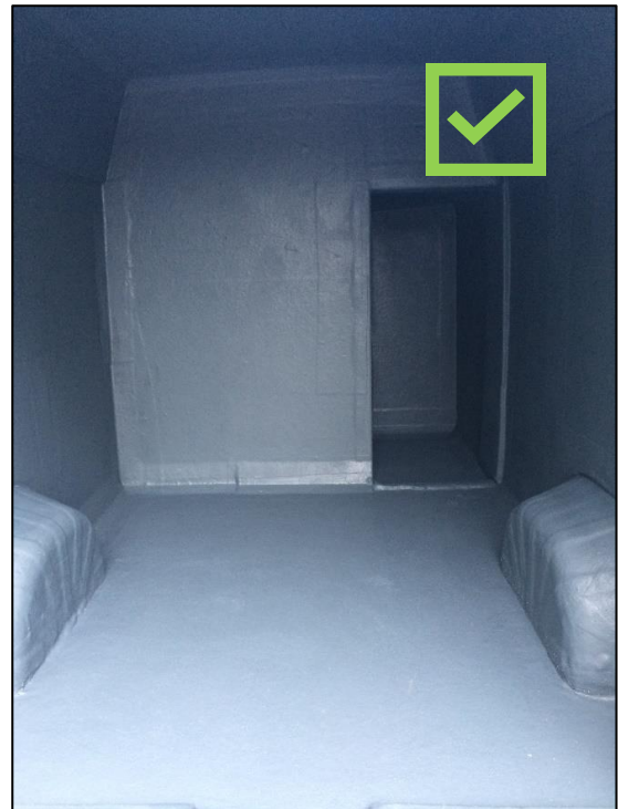
2. Entire van compartment sealed and segregated from top to bottom, rounded wheel arch edges to minimise risk of bag puncture [Not shown but there should be a secondary door to protect the door furniture, rear electrical lights and prevent waste falling out on opening]
