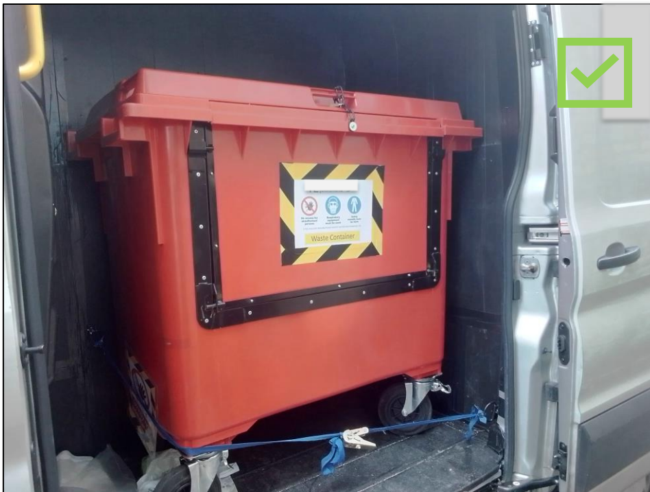
5. Wheelie bin signed and secured in side compartment of van
