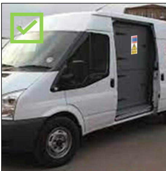
3. Side access compartment fitted with a secondary door which is signed and lockable
